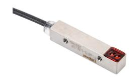
ProSense photoelectric sensor, rectangular, die-cast zinc, diffuse with background suppression, 5-30mm sensing distance, light-on, NPN, 500 Hz switching frequency, 0.6ft/0.2m cable length, 3-pin M8 quick-disconnect.
