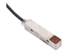
ProSense photoelectric sensor, rectangular, die-cast zinc housing, through-beam receiver, 0-2.2m sensing distance, 10-30 VDC operating voltage, dark-on, PNP, 3-wire, 3-pin M8 quick-disconnect.
