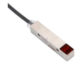
ProSense photoelectric sensor, rectangular, polarized retroreflective, visible red, 0-1m sensing distance, dark-on, PNP, 3-wire, 3-pin M8 quick-disconnect.
