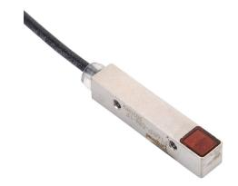
ProSense photoelectric sensor, rectangular, polarized retroreflective, visible red, 0-1m sensing distance, dark-on, NPN, 3-wire, 3-pin M8 quick-disconnect.
