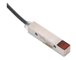
ProSense photoelectric sensor, rectangular, die-cast zinc housing, through-beam emitter, visible red light emission, 0-2.2m sensing distance, 10-30 VDC operating voltage, 2-wire, 3-pin M8 quick-disconnect.
