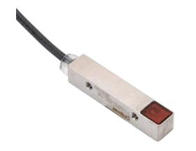
ProSense photoelectric sensor, rectangular, die-cast zinc housing, through-beam emitter, visible red, 0-2.2m sensing distance, 10-30 VDC operating voltage, 2-wire, 3-pin M8 quick-disconnect.
