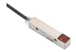
ProSense photoelectric sensor, rectangular, diffuse, visible red, 1-60mm sensing distance, light-on, PNP, 500 Hz switching frequency, die-cast zinc housing, 3-pin M8 quick-disconnect.
