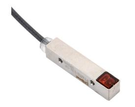
ProSense photoelectric sensor, rectangular, diffuse, visible red, 1-60mm sensing distance, light-on, NPN, 500 Hz switching frequency, die-cast zinc housing, 3-pin M8 quick-disconnect.
