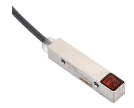
ProSense photoelectric sensor, rectangular, diffuse, visible red light emission, 1-60mm sensing distance, light-on, NPN, 500 Hz switching frequency, die-cast zinc housing, 3-pin M8 quick-disconnect.
