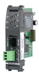
DirectLOGIC DL05/06 communication module, ASCII, 3 ports, buffered, 128k program memory, 100 MHz maximum switching frequency, (2) RS-232 and (1) RS-485 port(s). For use with DL05 and DL06 PLCs.
