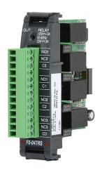
DirectLOGIC DL05/06 relay output module, 4-point, 6-48 VDC/6-208 VAC, (2) Form A, (2) Form C, 4 isolated common(s), 1 point(s) per common, 3A/point. Removable terminal block included.
