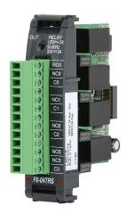
DirectLOGIC DL05/06 relay output module, 4-point, 6-48 VDC/6-208 VAC, (2) Form A, (2) Form C, 4 isolated common(s), 1 point(s) per common, 3A/point. Removable terminal block included.
