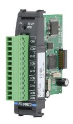
DirectLOGIC DL05/06 temperature input module, RTD, 4-channel, 16-bit resolution, input RTD type(s): Pt100, Pt1000, JPt100, Cu10, Cu25 and Ni120.
