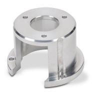
Koyo round mounting flange, 1.86in bolt hole circle, (1.34in height), metal. For use with Koyo TRDA-2E series encoders. Flange and encoder mounting hardware included.
