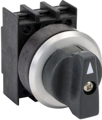
Schmersal selector switch, IP65, 30mm, 3-position, spring return to center from right or left, operator only, plastic base, metal bezel, Operator: black, knob, 29.5mm, round, plastic. Requires contact blocks.
