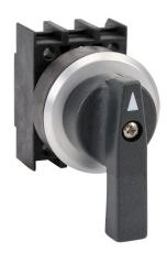
Schmersal selector switch, IP65, 30mm, 3-position, spring return to center from right or left, operator only, plastic base, metal bezel, Operator: black, lever, 29.5mm, round, plastic. Requires contact blocks.
