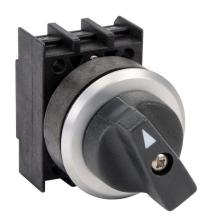
Schmersal selector switch, IP65, 30mm, 2-position, spring return from right, operator only, plastic base, metal bezel, Operator: black, knob, 29.5mm, round, plastic. Requires contact blocks.
