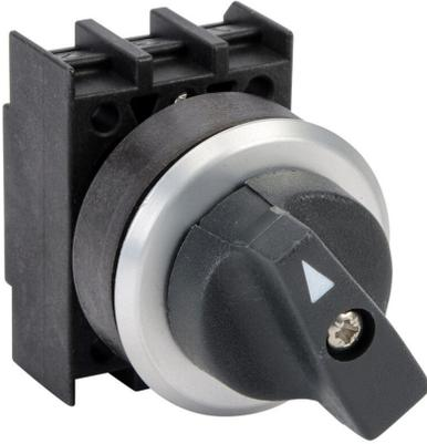
Schmersal selector switch, IP65, 30mm, 3-position, maintained, operator only, plastic base, metal bezel, Operator: black, knob, 29.5mm, round, plastic. Requires contact blocks.
