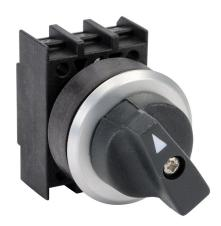
Schmersal selector switch, IP65, 30mm, 3-position, maintained, operator only, plastic base, metal bezel, Operator: black, knob, 29.5mm, round, plastic. Requires contact blocks.
