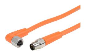
AutomationDirect connection cable, M8 axial male to right-angle female, 4-pole, PVC jacket, orange, 16.4ft/5m cable length, IP65, IP67, IP68 and IP69K, suitable for food and beverage applications.
