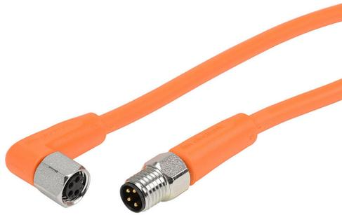
AutomationDirect connection cable, M8 axial male to right-angle female, 4-pole, PVC jacket, orange, 6.5ft/2m cable length, IP65, IP67, IP68 and IP69K, suitable for food and beverage applications.
