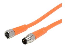
AutomationDirect connection cable, M8 axial female to axial male, 4-pole, PVC jacket, orange, 1.9ft/0.6m cable length, IP65, IP67, IP68 and IP69K, suitable for food and beverage applications.
