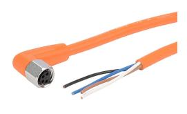
AutomationDirect connection cable, M8 right-angle female to pigtail, 4-pole, PVC jacket, orange, 32.8ft/10m cable length, IP65, IP67, IP68 and IP69K, suitable for food and beverage applications.
