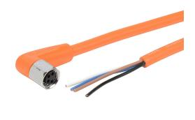
AutomationDirect connection cable, M8 right-angle female to pigtail, 4-pole, PVC jacket, orange, 16.4ft/5m cable length, IP65, IP67, IP68 and IP69K, suitable for food and beverage applications.
