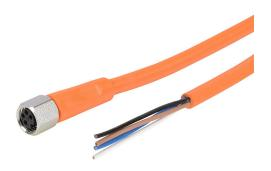
AutomationDirect connection cable, M8 axial female to pigtail, 4-pole, PVC jacket, orange, 32.8ft/10m cable length, IP65, IP67, IP68 and IP69K, suitable for food and beverage applications.
