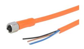
AutomationDirect connection cable, M8 axial female to pigtail, 4-pole, PVC jacket, orange, 6.5ft/2m cable length, IP65, IP67, IP68 and IP69K, suitable for food and beverage applications.
