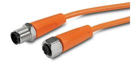
AutomationDirect connection cable, M12 axial female to axial male, 4-pole, PVC jacket, orange, 16.4ft/5m cable length, IP67, IP68 and IP69K, suitable for food and beverage applications.
