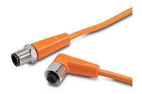
AutomationDirect connection cable, M12 right-angle female to axial male, 4-pole, PVC jacket, orange, 6.5ft/2m cable length, IP67, IP68 and IP69K, suitable for food and beverage applications.
