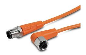
AutomationDirect connection cable, M12 right-angle female to axial male, 4-pole, PVC jacket, orange, 3.2ft/1m cable length, IP67, IP68 and IP69K, suitable for food and beverage applications.
