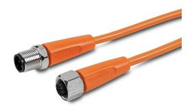
AutomationDirect connection cable, M12 axial female to axial male, 4-pole, PVC jacket, orange, 1.9ft/0.6m cable length, IP67, IP68 and IP69K, suitable for food and beverage applications.
