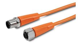
AutomationDirect connection cable, M12 axial female to axial male, 4-pole, PVC jacket, orange, 1.9ft/0.6m cable length, IP67, IP68 and IP69K, suitable for food and beverage applications.
