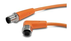
AutomationDirect connection cable, M12 right-angle female to axial male, 4-pole, PVC jacket, orange, 0.9ft/0.3m cable length, IP67, IP68 and IP69K, suitable for food and beverage applications.
