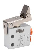
NITRA manual valve, 2-port (3-way), 2-position, N.C., metal plunger with one-way metal roller, spring return, side ports, (1) 5/32in (4mm) PTC tubing inlet(s), (1) 5/32in (4mm) PTC tubing outlet(s), (1) vent hole exhaust(s), Cv=0.13.
