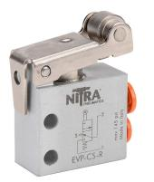
NITRA pneumatic manual valve, 2-port (3-way), 2-position, N.C., roller lever, spring return, side ports, (1) 5/32in (4mm) push-to-connect inlet(s), (1) 5/32in (4mm) push-to-connect outlet(s), (1) vent hole exhaust(s), Cv=0.13.
