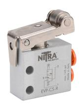
NITRA manual valve, 2-port (3-way), 2-position, N.C., metal plunger with metal roller, spring return, side ports, (1) 5/32in (4mm) PTC tubing inlet(s), (1) 5/32in (4mm) PTC tubing outlet(s), (1) vent hole exhaust(s), Cv=0.13.
