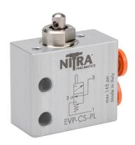
NITRA pneumatic manual valve, 2-port (3-way), 2-position, N.C., metal plunger, spring return, side ports, (1) 5/32in (4mm) push-to-connect inlet(s), (1) 5/32in (4mm) push-to-connect outlet(s), (1) vent hole exhaust(s), Cv=0.13.
