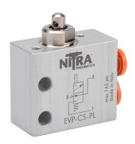
NITRA manual valve, 2-port (3-way), 2-position, N.C., metal plunger, spring return, side ports, (1) 5/32in (4mm) PTC tubing inlet(s), (1) 5/32in (4mm) PTC tubing outlet(s), (1) vent hole exhaust(s), Cv=0.13.
