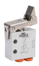
NITRA pneumatic manual valve, 2-port (3-way), 2-position, N.C., unidirectional roller lever, spring return, axial ports, (1) 5/32in (4mm) push-to-connect inlet(s), (1) 5/32in (4mm) push-to-connect outlet(s), (1) vent hole exhaust(s), Cv=0.13.
