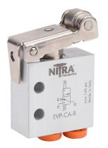
NITRA pneumatic manual valve, 2-port (3-way), 2-position, N.C., roller lever, spring return, axial ports, (1) 5/32in (4mm) push-to-connect inlet(s), (1) 5/32in (4mm) push-to-connect outlet(s), (1) vent hole exhaust(s), Cv=0.13.
