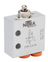
NITRA pneumatic manual valve, 2-port (3-way), 2-position, N.C., metal plunger, spring return, axial ports, (1) 5/32in (4mm) push-to-connect inlet(s), (1) 5/32in (4mm) push-to-connect outlet(s), (1) vent hole exhaust(s), Cv=0.13.
