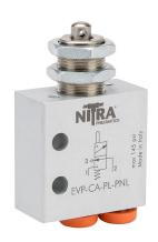
NITRA pneumatic manual valve, 2-port (3-way), 2-position, N.C., metal plunger, spring return, axial ports, (1) 5/32in (4mm) push-to-connect inlet(s), (1) 5/32in (4mm) push-to-connect outlet(s), (1) vent hole exhaust(s), Cv=0.13, through panel mount.
