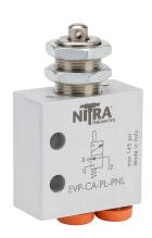
NITRA manual valve, 2-port (3-way), 2-position, N.C., metal plunger, spring return, axial ports, (1) 5/32in (4mm) PTC tubing inlet(s), (1) 5/32in (4mm) PTC tubing outlet(s), (1) vent hole exhaust(s), Cv=0.13, through panel mount.
