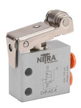
NITRA pneumatic manual valve, 2-port (3-way), 2-position, N.O., roller lever, spring return, side ports, (1) 5/32in (4mm) push-to-connect inlet(s), (1) 5/32in (4mm) push-to-connect outlet(s), (1) vent hole exhaust(s), Cv=0.13.
