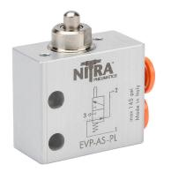
NITRA pneumatic manual valve, 2-port (3-way), 2-position, N.O., metal plunger, spring return, side ports, (1) 5/32in (4mm) push-to-connect inlet(s), (1) 5/32in (4mm) push-to-connect outlet(s), (1) vent hole exhaust(s), Cv=0.13.
