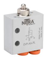
NITRA pneumatic manual valve, 2-port (3-way), 2-position, N.O., metal plunger, spring return, axial ports, (1) 5/32in (4mm) push-to-connect inlet(s), (1) 5/32in (4mm) push-to-connect outlet(s), (1) vent hole exhaust(s), Cv=0.13.
