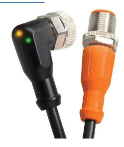
AutomationDirect connection cable, M12 right-angle female to axial male, 4-pole, 10-36 VDC, PNP LED, PUR jacket, black, 32.8ft/10m cable length, IP67, IP68 and IP69K.
