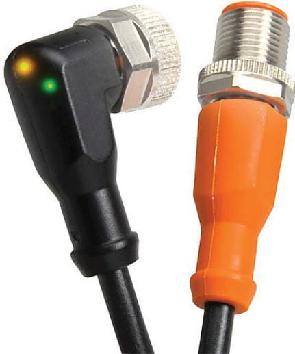
AutomationDirect connection cable, M12 right-angle female to axial male, 4-pole, 10-36 VDC, PNP LED, PUR jacket, black, 3.2ft/1m cable length, IP67, IP68 and IP69K.
