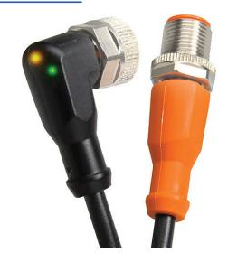
AutomationDirect connection cable, M12 right-angle female to axial male, 4-pole, 10-36 VDC, PNP LED, PUR jacket, black, 1.9ft/0.6m cable length, IP67, IP68 and IP69K.
