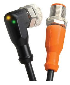
AutomationDirect connection cable, M12 right-angle female to axial male, 4-pole, 10-36 VDC, PNP LED, PUR jacket, black, 0.9ft/0.3m cable length, IP67, IP68 and IP69K.
