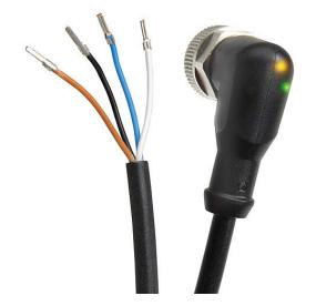
AutomationDirect connection cable, M12 right-angle female to pigtail, 4-pole, 10-36 VDC, PNP LED, PUR jacket, black, 32.8ft/10m cable length, IP67, IP68 and IP69K.
