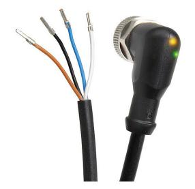
AutomationDirect connection cable, M12 right-angle female to pigtail, 4-pole, 10-36 VDC, PNP LED, PUR jacket, black, 6.5ft/2m cable length, IP67, IP68 and IP69K.
