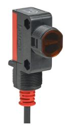
Leuze photoelectric sensor, rectangular, diffuse, visible red light emission, 1-650mm sensing distance, complementary light-on/dark-on, PNP, teach-in button, 500 Hz switching frequency, ABS plastic housing, pigtail.
