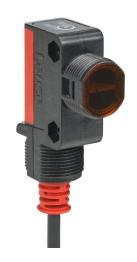
Leuze photoelectric sensor, rectangular, diffuse, visible red, 1-650mm sensing distance, complementary light-on/dark-on, PNP, teach-in button, 500 Hz switching frequency, ABS plastic housing, pigtail.
