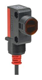
Leuze photoelectric sensor, rectangular, diffuse, visible red, 1-650mm sensing distance, complementary light-on/dark-on, PNP, teach-in button, 500 Hz switching frequency, ABS plastic housing, 4-pin M12 quick-disconnect.
