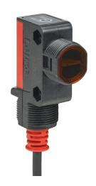
Leuze photoelectric sensor, rectangular, diffuse, visible red light emission, 1-650mm sensing distance, complementary light-on/dark-on, NPN, teach-in button, 500 Hz switching frequency, ABS plastic housing, pigtail.
