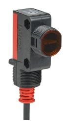
Leuze photoelectric sensor, rectangular, diffuse, visible red light emission, 1-650mm sensing distance, complementary light-on/dark-on, NPN, teach-in button, 500 Hz switching frequency, ABS plastic housing, 4-pin M12 quick-disconnect.
