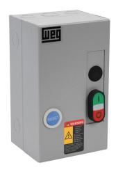
WEG Electric ESWS series manual motor starter, pushbutton, 25A, 2-pole, 120 VAC (50/60Hz) coil voltage, thermal overload, 15.0-23.0.A Adjustable, NEMA 1.
