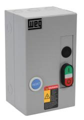
WEG Electric ESWS series manual motor starter, pushbutton, 12A, 2-pole, 120 VAC (50/60Hz) coil voltage, thermal overload, 8.0-12.5A Adjustable, NEMA 1.
