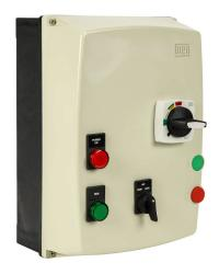
WEG Electric ESWE series combination Type-E motor starter, 9A, 3-pole, 480 VAC (50/60Hz) coil voltage, bi-metallic, 1.0–1.6A adjustable, 21A instantaneous trip rating, NEMA 4/4X.
